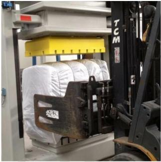
The last component in the processing line is a vertical bale press, especially designed and built for the packaging process.
